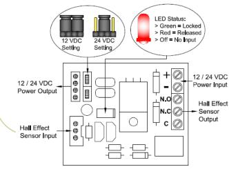
**IMPORTANT!** Set the jumper position according to the power input correctly before switch ON the power.
