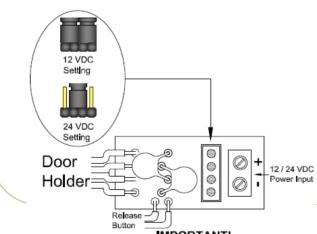
MPORTANT! Set the jumper position according to the power Input correctly before switch ON the power.
